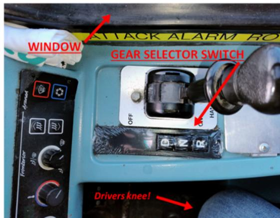
The offending gear selector switch – now covered in a waterproof film.
